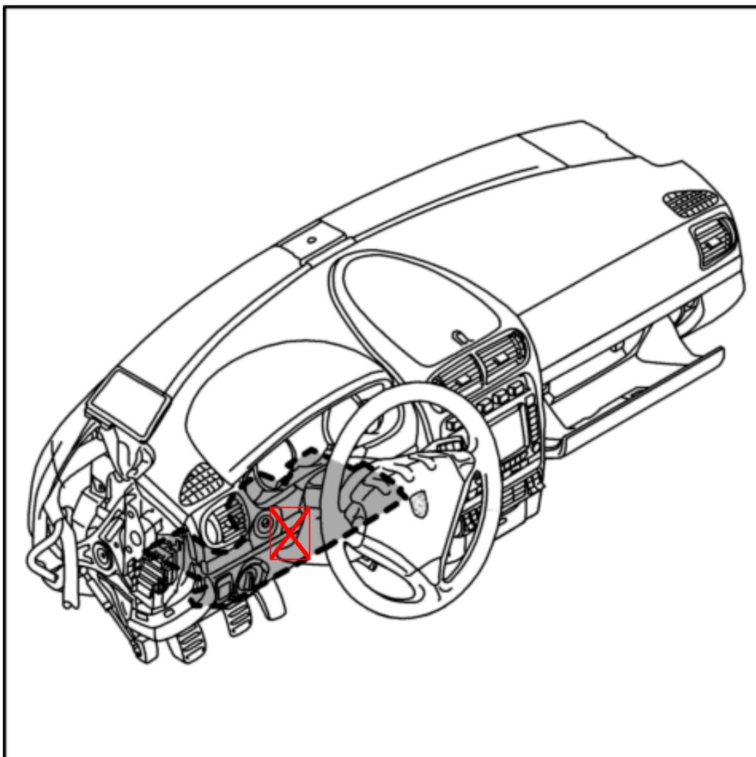
1. Insert cover under dashboard on the driver's side
