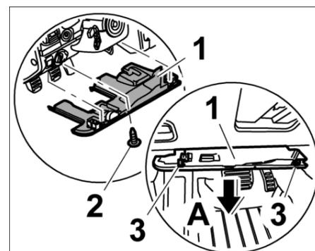
3. Disconnect the plug connections and remove cover under dashboard on the driver's side.
