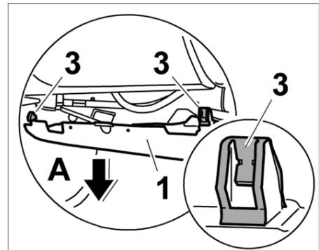
3. Disconnect the plug connections and remove cover under dashboard on the passenger's side.
