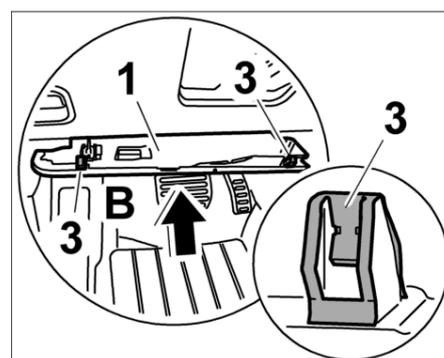
**Installing cover under dashboard on the passenger's side**
