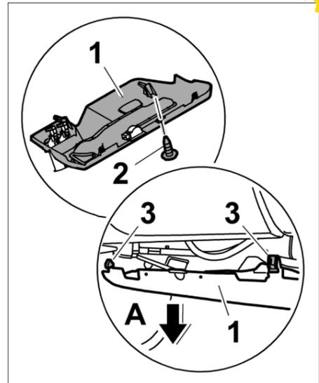
downwards until the plug connections are accessible -arrow A- .
