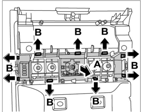
19. Engage the two covers at the back **-A-** and press in at the front edge **-arrow B-** until the locking tabs (three on each cover) are felt to engage **-C-**. Make sure that the covers are positioned correctly at the frame of the switch trims **-D-**.
