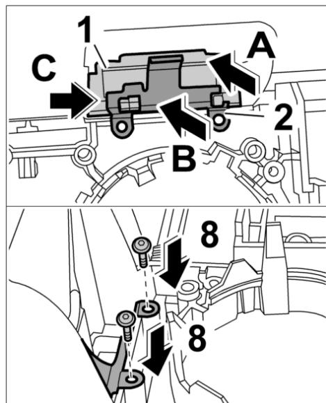
9. Press in the switch trims **-arrow A-** until you feel the locking tabs **-B-** engage.
