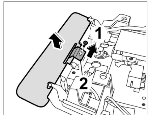
2. Unlock connector on garage door opener control unit **-arrows A-** and pull it off **-arrow B-**.
