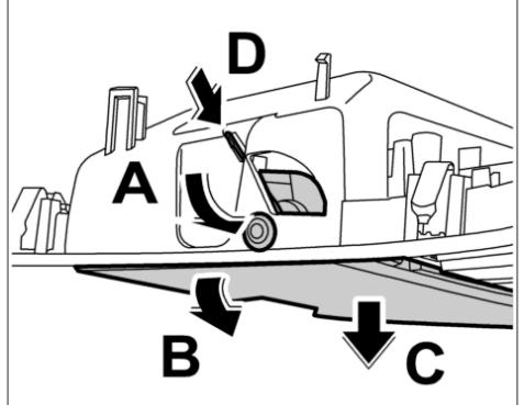
35. Pull off the bearing sleeve **-arrow A-** and remove the spring **-arrow B-**.
