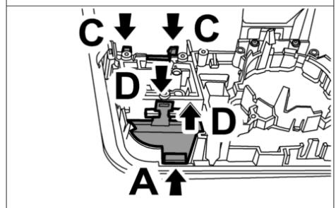
20. Insert the light ring into the cover and align the two markings **-arrow-**
