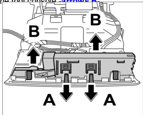
10. Unscrew the four fastening screws 4- and remove printed circuit board for interior lighting -arrow- .
