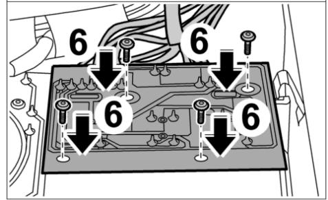
25. Turn the printed circuit board around **-arrow B-** and screw down with four fastening screws **-6-**.
