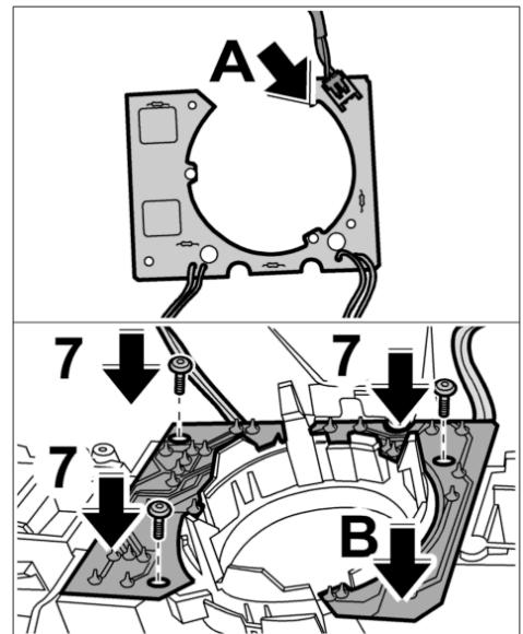
29. Place the printed circuit board in installation position **-arrow B-** and screw down with three fastening screws **-7-**.
