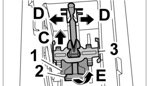
26. Remove the contact bridge **-1-** ( **-arrow C-** ).
