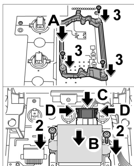
40. Push in connector **-arrow C-** until the locking tabs **-D-** are felt to engage.
