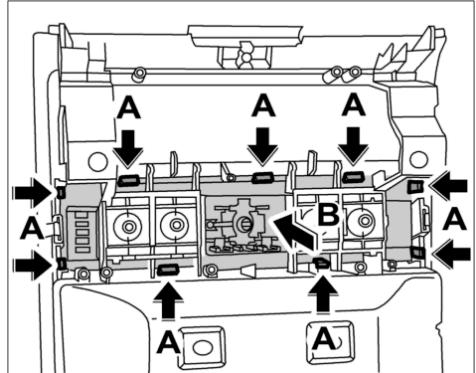
25. Press the clip together **-arrows A-** and carefully remove the spring **-arrow B-**.
