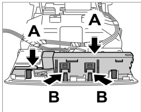
35. Attach the connector to the printed circuit board **-arrow A-** until it engages securely.
