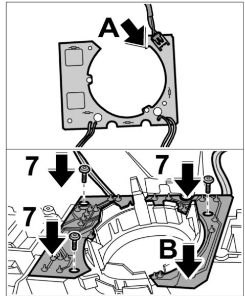
30. Insert the microphone **-arrow A-** until the two locking tabs **-B-** are felt to engage.
