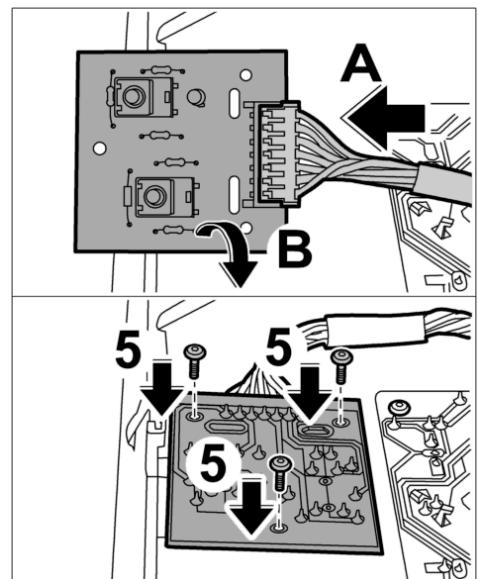
28. Connect the connector to the printed circuit board until they engage securely **-arrow A-**.
