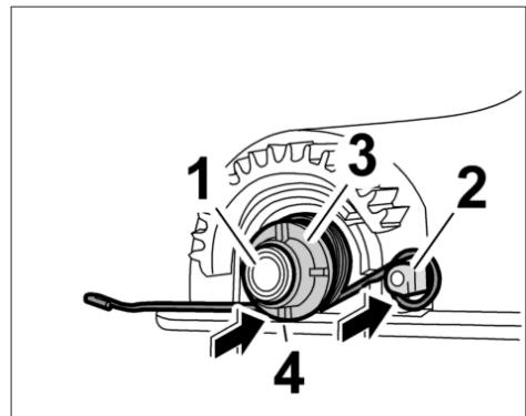
2. Connect the bearing sleeve with the contact surface **-3-** pointing towards the spring at the pivot axis. Make sure that the flat edge **-4-** of the contact surface is facing downwards.
