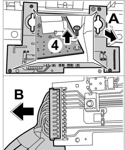
12. Press in the two clips -arrows A- and press the reading light out in a downward direction -arrow B- .
