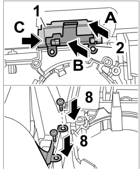
8. Insert the spring **-2-** ( **-arrow B-** ), move it to the right **-arrow C-** , and screw down using the two fastening screws **-8-** .
