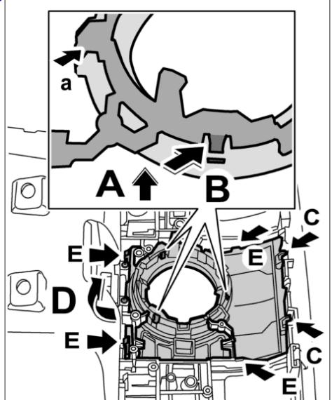
22. Engage the cover at the roof console **-C-** and press it in **-arrow D-** until the four locking tabs **-E-** are felt to engage.
