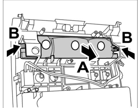
32. Place the switch in installation position and press it in carefully **-arrow A-**. Make sure that all three locking hooks **-B-** engage at the switch.
