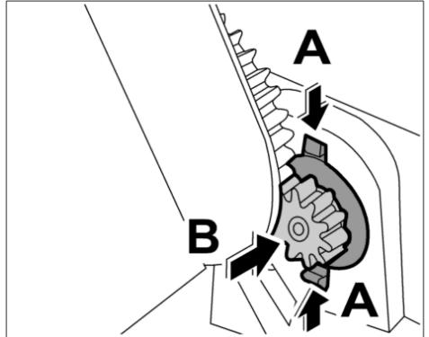
34. Press the right bearing pin at the edge inwards **-arrow A- -arrow A-**, pivot the shelf down **-arrow B-** and remove it **-arrow C-**. Push the spring through the opening at the same time **-arrow D-**.
