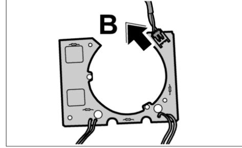
19. Remove the printed circuit board (sun blind) **-arrow A-** and pull off the connector **-arrow B-** .
