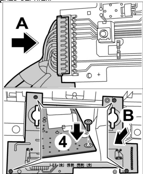
36. Place the printed circuit board in installation position **-arrow B-** and screw down with four fastening screws **-4-**.
