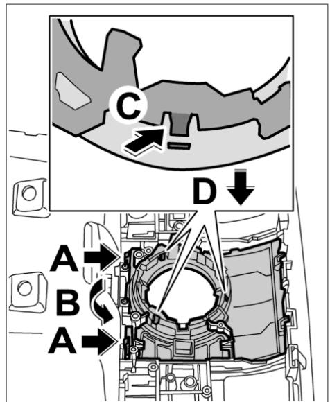
23. Release the nine locking tabs **-arrows A-** and press the two covers down and out **-arrows B-**.
