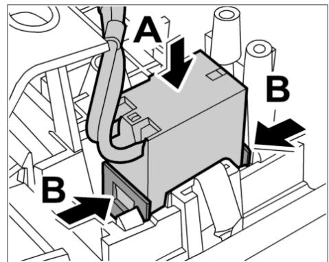
31. Place the reading light in installation position and press it in **-arrow A-** until the two clips **-B-** engage securely.
