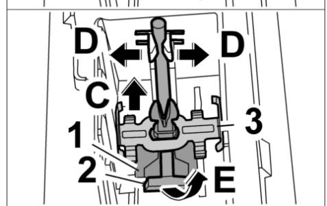
27. Carefully pull the holder out of the locking mechanism **-2-** ( **-arrows D-** ) and pull the switch **-3-** down and out **-arrow E-** .
