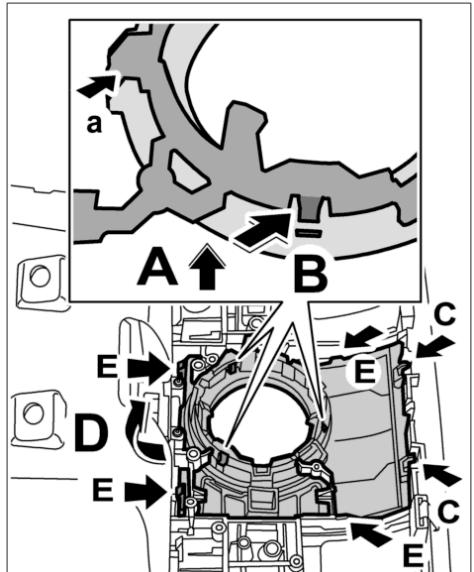
23. Insert the wiring harness into the brackets **-arrow-**.
