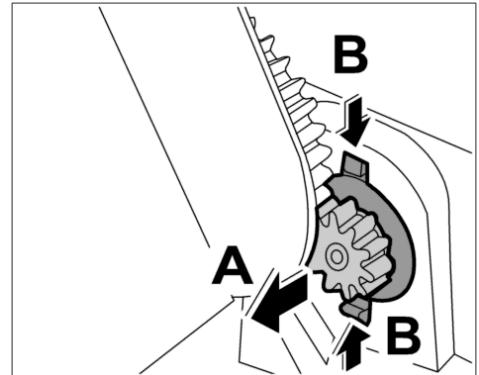
7. Place the push-button **-1-** in installation position **-arrow A-**.
