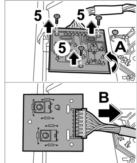
15. Turn the printed circuit board **-arrow A-** and pull the connector off the printed circuit board (P- & SOS button) **-arrow B-**.
