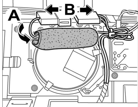
8. Carefully pull the three locking tabs **-A-** apart and pull the switch up and out **-B-**.
