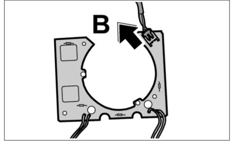
20. Remove the wiring harness from the brackets **-arrows-** .
