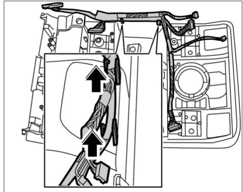
21. Release the cover **-arrows A-** and unfold it downwards **-arrow B-** .
