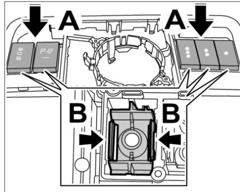
10. Press the bracket carefully to the inside **-arrow A-**.
