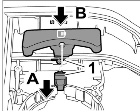
11. Place the switch trim in installation position and press it in **-arrow B-** until it engages securely in the retaining pivot **-1-**.
