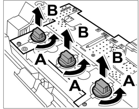
6. Pull the piece of plastic foam off the plug connection **-arrow A-**.
