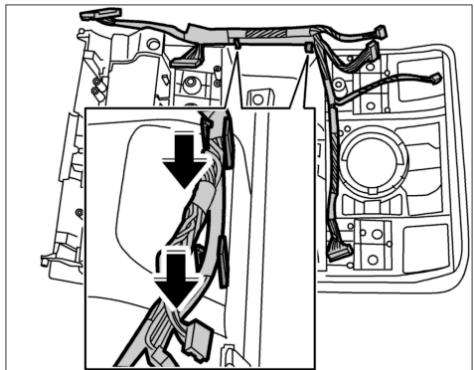
24. Connect the two connectors on the printed circuit board until they are felt to engage **-arrows A-**.
