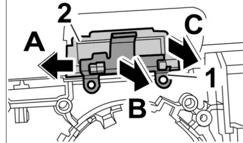
31. Move spring **-1-** for the push-button **-2-** to the left **-arrow A-** and remove it **-arrow B-** .
