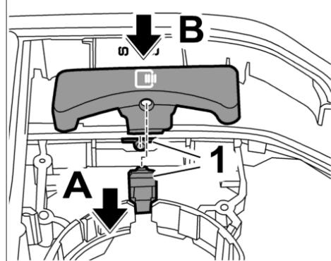
13. Position the sliding switch **-1-** in the cover in such a way that the pictogram is aligned with that on the adjacent switch trims **-2-**.
