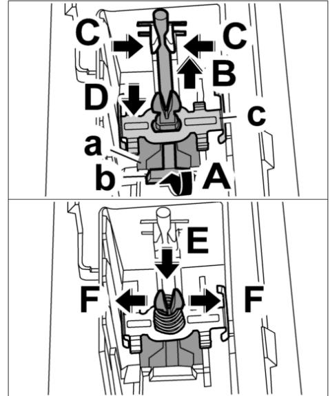
16. Connect the contact bridge **-c-** to the switch **-arrow D-** .
