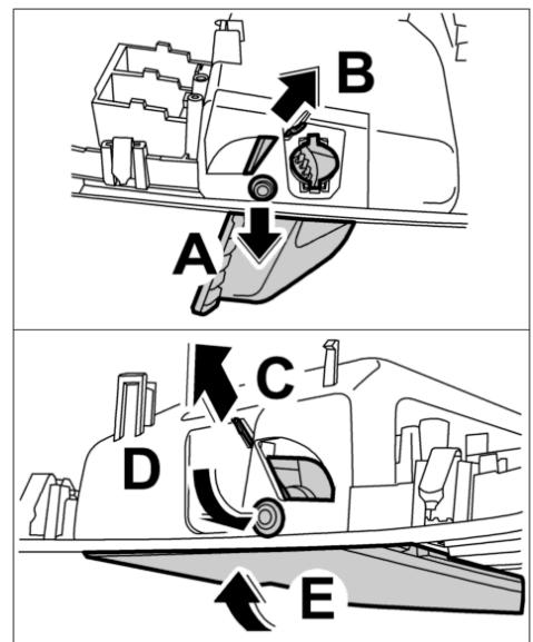
6. Press in the closing damper **-arrow A-** until you feel the locking tabs **-B-** engage.
