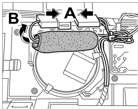
34. Insert the sensor into the roof console frame **-A-** until the two locking hooks **-B-** are felt to engage. Ensure it is seated properly.
