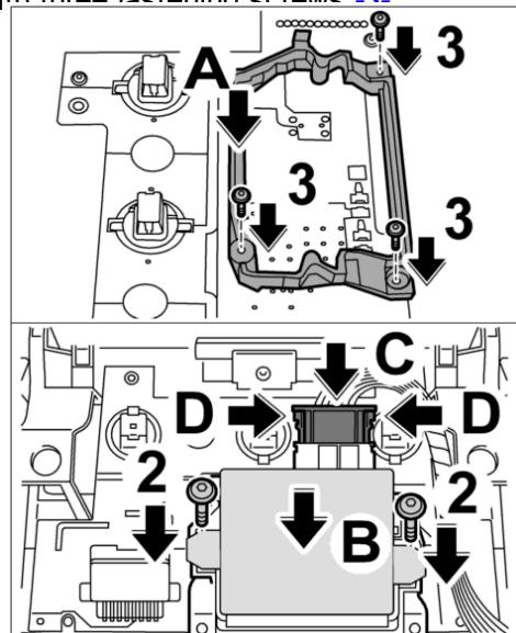
39. Place the control unit on the holder **-arrow B-** and screw down with both fastening screws **-2-**.
