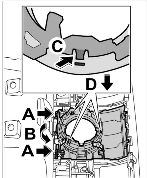
22. Release the lighting unit **-arrow C-** and press it down and out **-arrow D-** .
