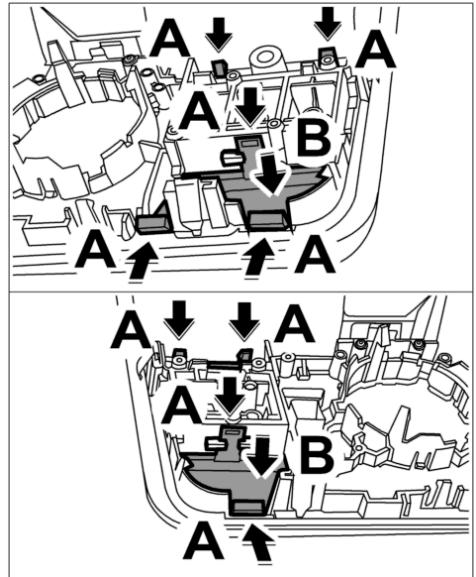
24. Release the nine locking tabs **-arrows A-** and carefully press the cover down and out **-arrow B-**.
