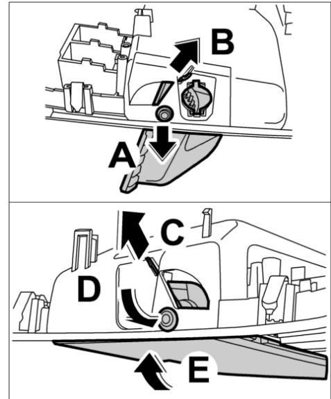
5. Press in the bearing pin at the underside **-arrow D-**, then press the shelf into the roof console **-arrow E-** until the bearing pin with the bearing sleeve engages securely.
