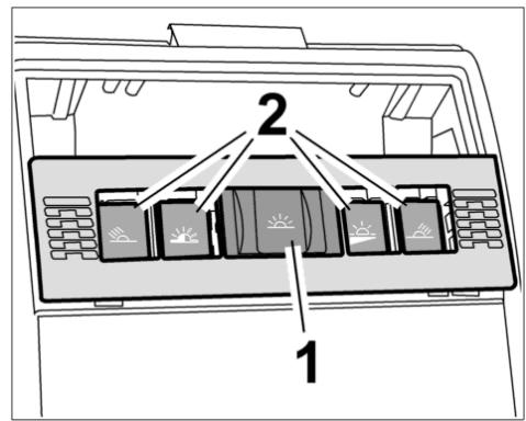
15. Insert the holder **-1-** through the sliding switch **-2-** ( **-arrow A-** ) and press it carefully into the bracket **-arrow B-** until the locking tabs are felt to engage **-C-** .
