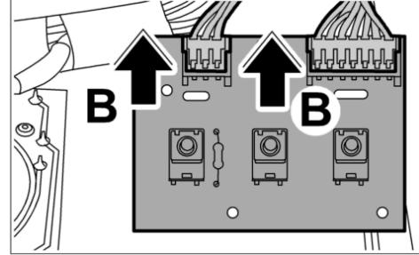
17. Turn the printed circuit board (garage door opener) **-arrow A-** and pull the two connectors off the printed circuit board **-arrows B-** .
