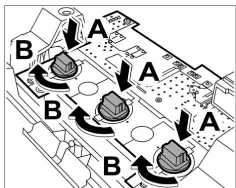
37. Insert bulbs into the printed circuit board **-arrow A-** and tighten **-arrow B-**.
