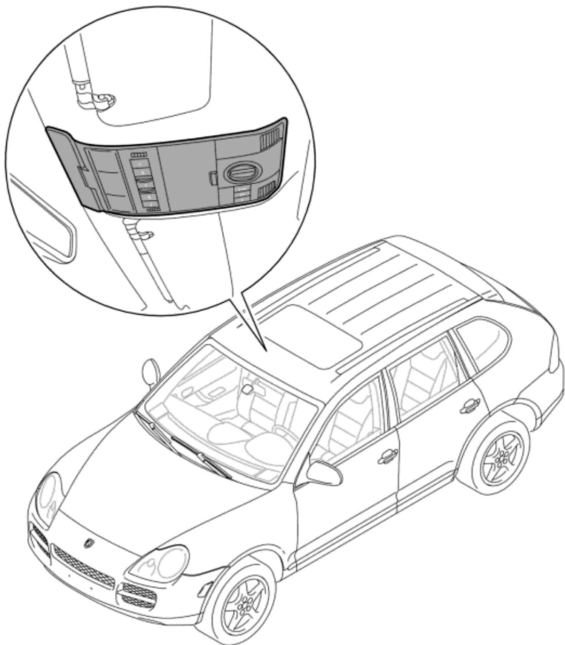
Remove front roof console. → 601219 Removing and installing switch for sunroof - section on "Removing"
