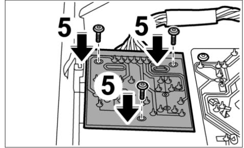
27. Turn the printed circuit board around **-arrow B-** and screw down with three fastening screws **-5-**.
