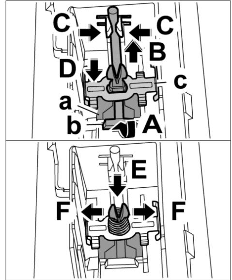
17. Connect the spring to the sliding switch **-a-** ( **-arrow E-** ) until the locking tabs are felt to engage **-arrows F-** .
