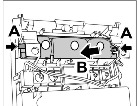
13. Release the microphone holder using a small screwdriver **-arrows A-** and remove the microphone **-arrow B-**.
