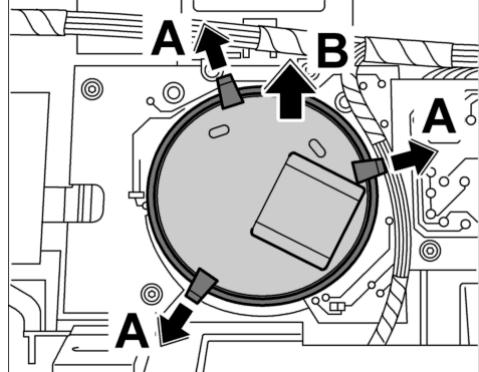
9. Release sensor for interior monitoring -arrows A- and remove it from the roof console -arrow B-.
