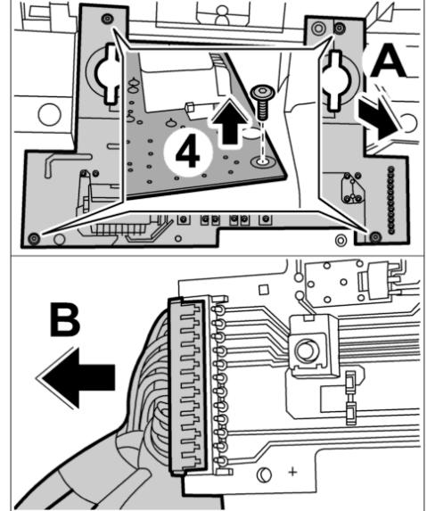
11. Carefully pull the connector off the printed circuit board -arrow B- .
