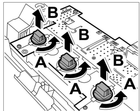
5. Turn the sockets of the bulbs for interior lighting to the left **-arrow A-** and remove them **-arrow B-**.
