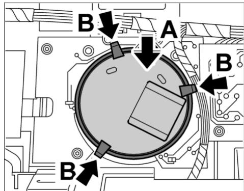
33. Connect the plug connection **-arrows A-** and slide the piece of plastic foam over the plug connection **-arrow B-**.
