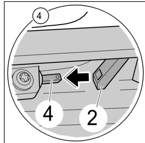
6.2. Push bellows **-2-** at the bottom in the rear area backwards into the guide.
