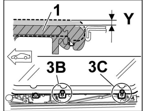
4. Tighten fastening screw M5 **-3B-** to specified tightening torque. → **Tightening torque: 4.5 (3.5 ftlb.) Nm +/-0.5 (0.5 ftlb.) Nm**
