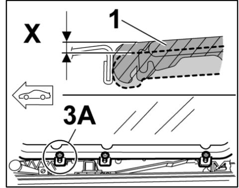
3. Adjust height **-Y-** of cover for sliding roof at rear → **Test and adjustment value: 0 mm +1 mm**
