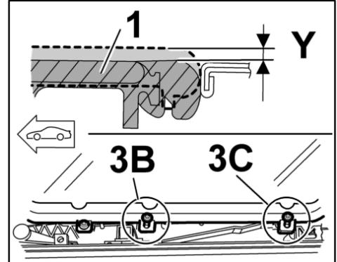
5. Tighten fastening screw M5 **-3C-** to specified tightening torque. → **Tightening torque: 4.5 (3.5 ftlb.) Nm +/-0.5 (0.5 ftlb.) Nm**
