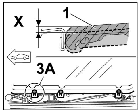
2. Tighten fastening screw M5 **-3A-** to specified tightening torque. → **Tightening torque: 4.5 (3.5 ftlb.) Nm +/-0.5 (0.5 ftlb.) Nm**
