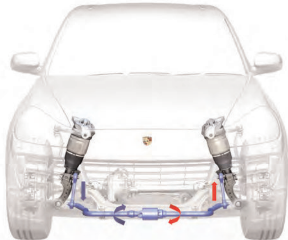
Principle for creating definable forces between body and wheel using active roll stabilization.
